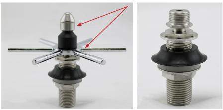
By unscrewing the <u>bottom nut</u> you can remove the <u>inner valve body</u>. Once the inner valve body has been removed it will expose the activation piston.
