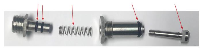
Insert the activation piston into the inner valve body, ensure that the spring is still sitting in the inner sleeve.
